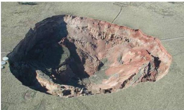
Fig. 1: Cave front at the Ridgeway mine eventually broke through to the surface.
