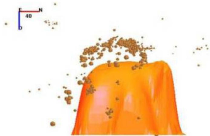
Fig. 2: Position of the cave based on borehole measurements compared to location of seismic events in fractured zone of the cave front.
