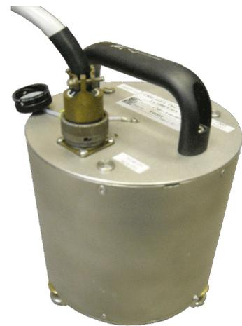
Fig. 2: Triaxial geophone installed to monitor hydroelectric dam reservoirs
