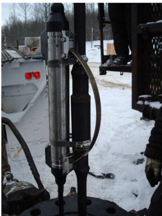
Fig. 1: ESG Bowspring sensor array is deployed
