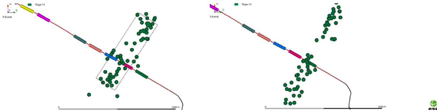
Fig. 2: Example of events from stage 14: (left) events locating out of zone using the initial velocity model and (right) events locating in-zone after the PSO method is applied to the data and the velocity model is adjusted to account for the geological structure between stages 9 and 10.
