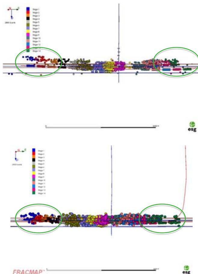
Fig. 3: Example of events for all stages of the fracture treatment: (top) before PSO is applied and (bottom) after PSO is applied
