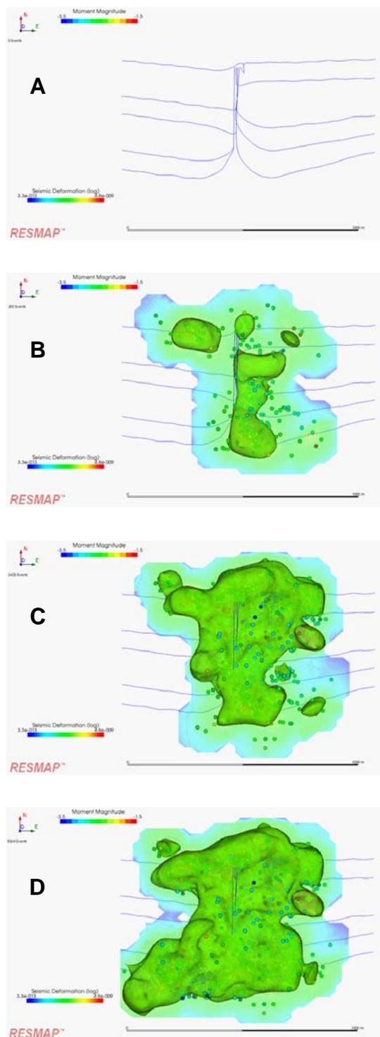
Fig. 2: Progression of a steam chamber using thermal methods for heavy oil production from 2002 to 2010.
