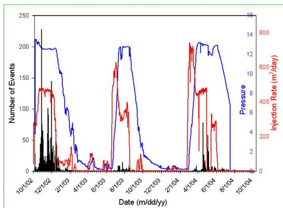
Fig. 4: Microseismic events and injection pressure
