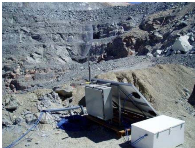
Fig. 3. Remote seismic station setup.
