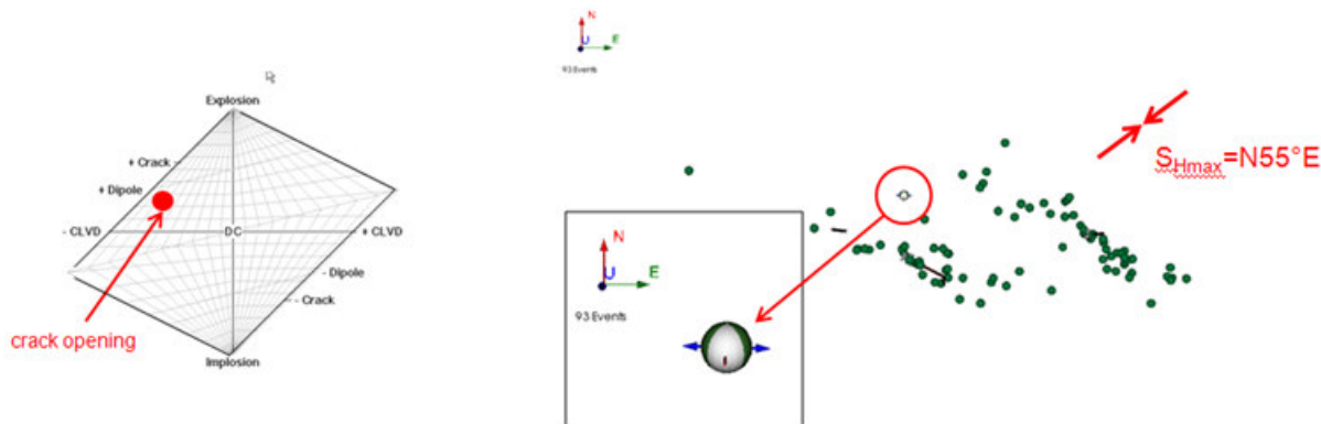
Figure 4: Seismic Moment Tensor Inversion (SMTI) Analysis indicates mechanism of failure consistent with a crack opening, and with potential failure planes oriented at N160°E or N24°E.
