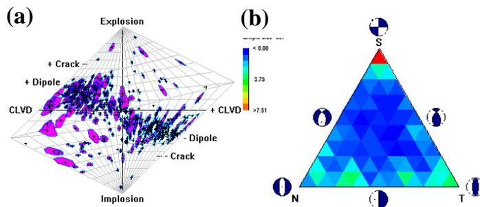
Fig. 4. Event mechanisms for the events around the East Stope on source mechanism (a) and faulting (b) type diagrams. Contours surrounding data points (crosses) in (a) correspond to one sigma interval for the respective estimates.
