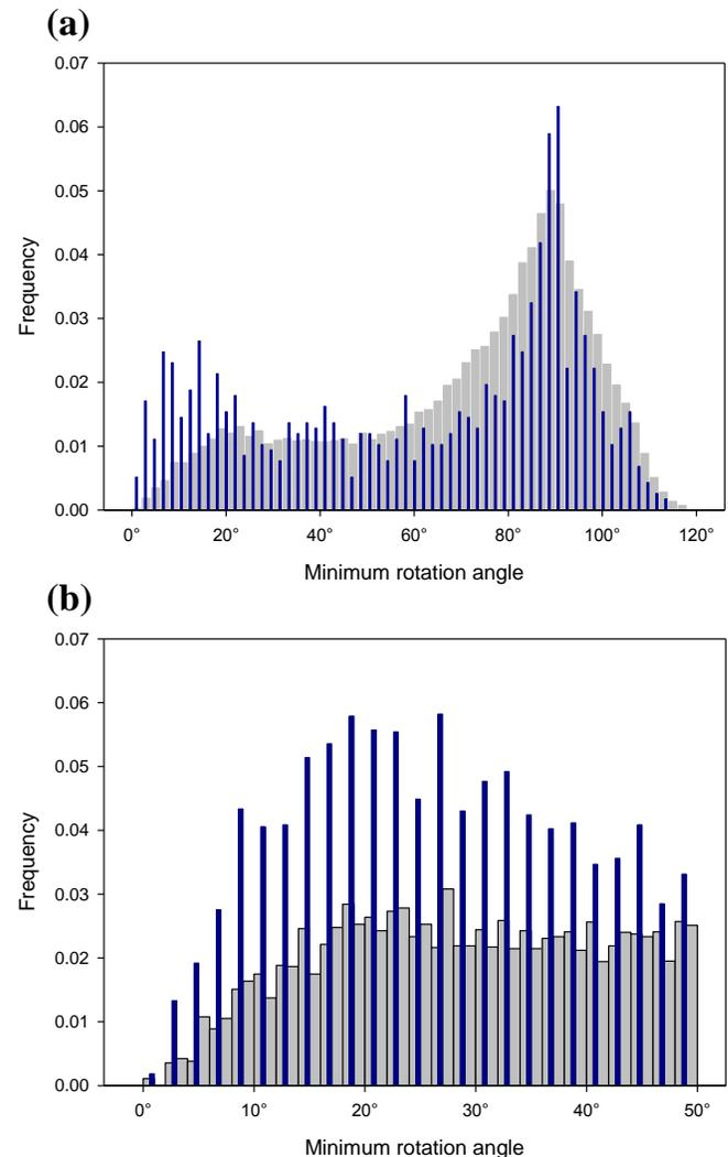
Fig. 7. Distribution of the minimum rotation angle for pair of mechanism solutions. The entire data sample is shown in gray. Dark blue bars correspond to pair events (a) separated by less than 5 m; and (b) separated by less than 24 hours.
