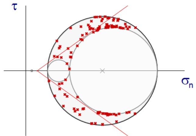
Fig. 6. Scaled Mohr diagram prior to April 21. Thin lines show Coulomb failure envelope with a friction angle of 36°.
