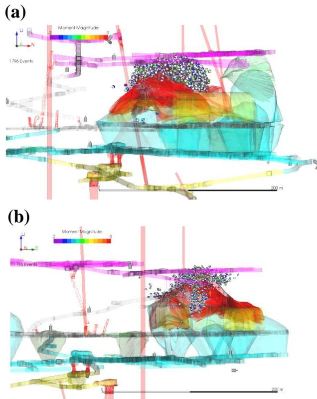
Fig. 3. Microseismic events with SMT solutions are located around the East Stope in (a) north-depth and (b) east-depth projections.
