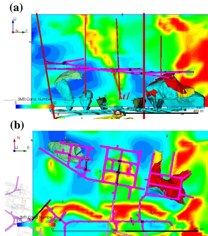
Fig. 2. Conditional number for SMT inversions, calculated over the study volume at 3D grid points in (a) north-east and (b) east-depth projections.
