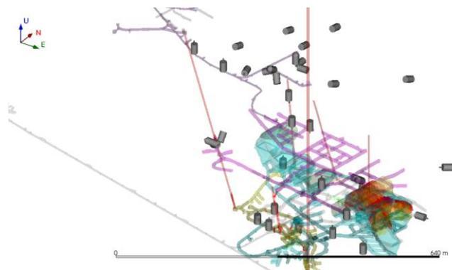
Fig. 1. Microseismic monitoring array at Goldex mine. Gray cylinders show the sensor locations.
