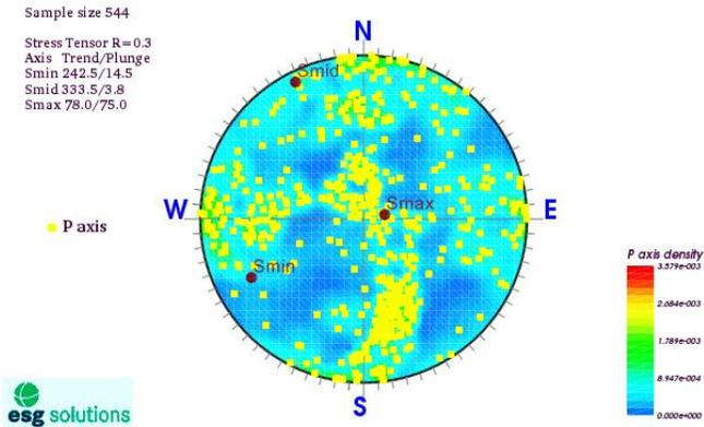
Fig. 5. Distribution of the SMT major double-couple P-axes around the East Stope, and the result of the ST inversion. Color refers to the probability density function.
