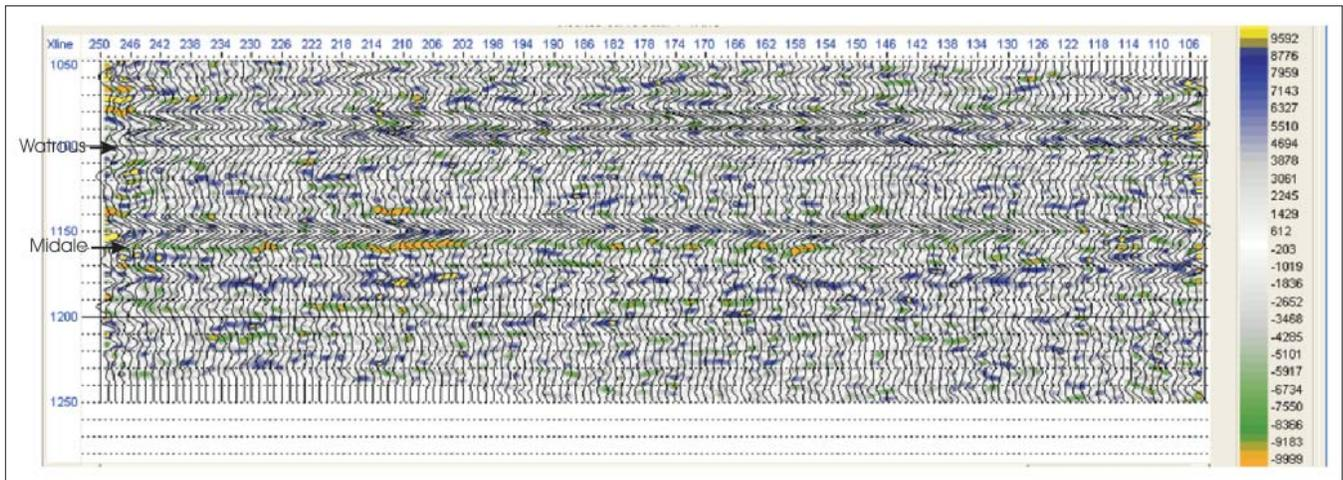
**Figure 4.** Time-lapse amplitude differences (2004 minus baseline data) are shown in color for a slice through the 3D difference volume. The baseline data are shown as a wiggle trace overlay (deflection to the right = positive amplitude). The top of the Watrous (seismic peak) and the Midale Marly (seismic trough) units are indicated. The vertical axis is two-way traveltime (ms), and the horizontal axis shows crossline numbers (10 crosslines constitute 400 m).
