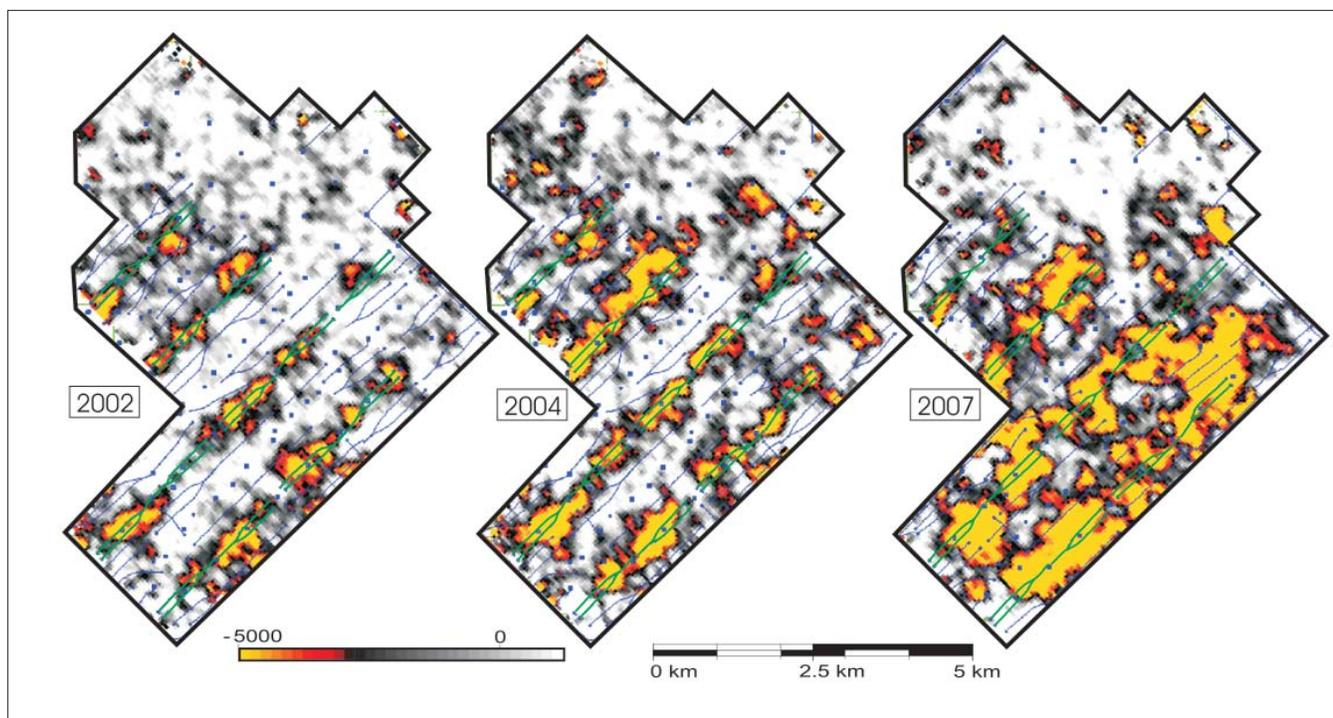
**Figure 5.** Time-lapse amplitude difference maps for the Midale Marly horizon. Only the negative amplitude differences are shown to accentuate CO<sub>2</sub> saturation effects. Dual-leg wells are either production (black) or CO<sub>2</sub> injection (green) wells.
