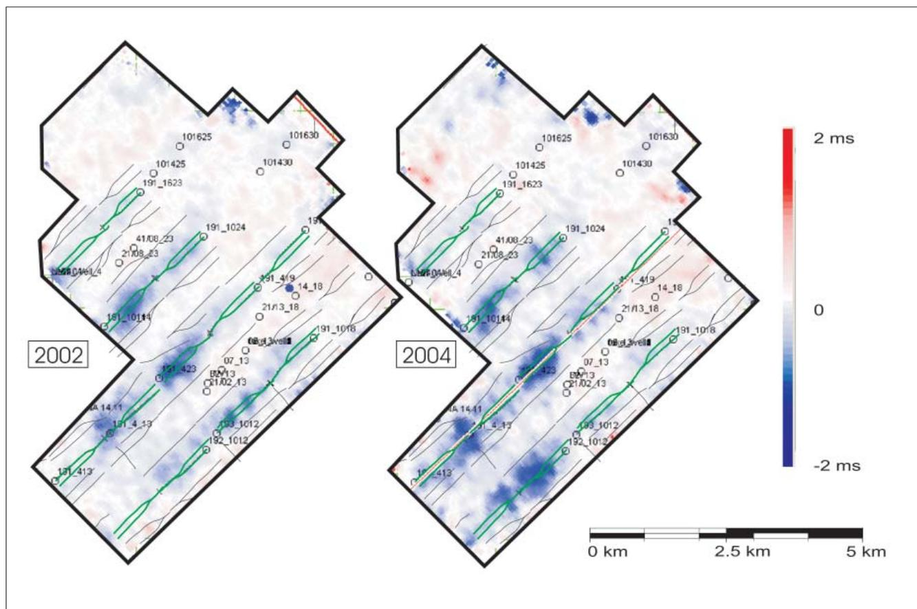
**Figure 6.** Time-lapse traveltim difference maps determined for a subreservoir horizon representing traveltim anomalies associated with propagation through the reservoir.
