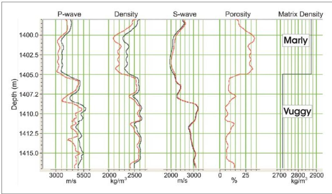
**Figure 3.** Log-based fluid substitution results calculated using the Gassmann equation. The original logs are shown in black, and logs with simulated CO<sub>2</sub> injection (substitution of brine by 30% brine and 70% CO<sub>2</sub>) are shown in red. The rock matrix properties used in this modeling were based on laboratory core-property measurements by Brown in 2002.
