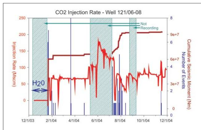
**Figure 7.** CO<sub>2</sub> injection rate, number of seismic events, and cumulative seismic moment versus time for a 12-month period starting 1 December 2003.
