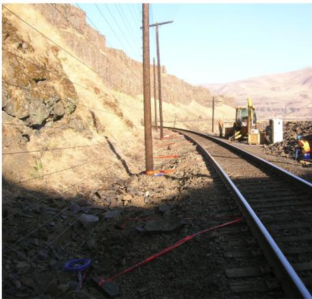
Fig. 1: Location of the seismic sensors (approximately in line with the hydro poles) in relation to the railway tracks and rock face
