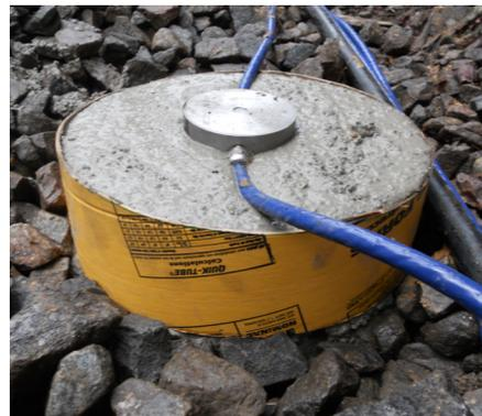
Fig. 2: Standard MRMS sensor installed near a railway track
