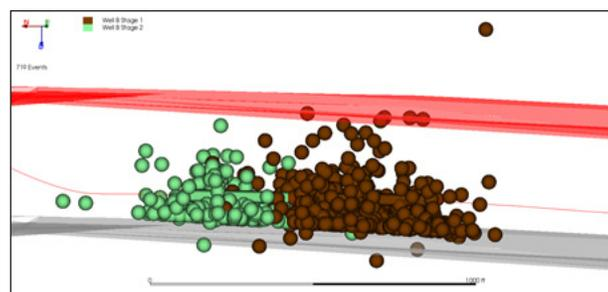
Fig 3: Cross-sectional view of microseismic events from 2 stages in Well B exhibiting vertical containment. The red and grey surfaces represent the top and bottom of the Marcellus, respectively.
