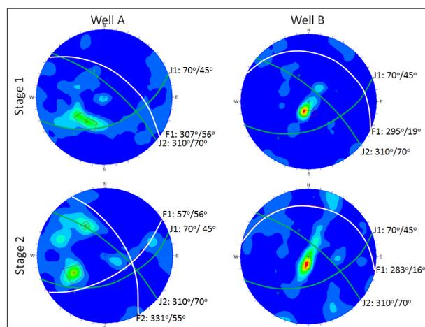
Figure 4: Lower stereographic projections of the poles to the SMTI-derived fracture planes in stages 1 and 2 of wells A and B respectively. These fracture planes are compared against the orientations of the dominant joint sets for the Marcellus described by Engelder et al. (2009).
