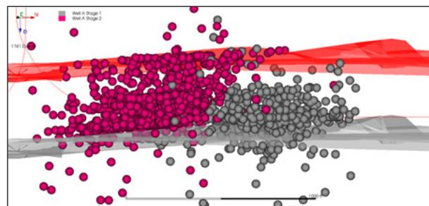
Fig 2: Cross-sectional view of microseismic events from 2 stages in Well A exhibiting significant vertical growth. The red and grey surfaces represent the top and bottom of the Marcellus, respectively.
